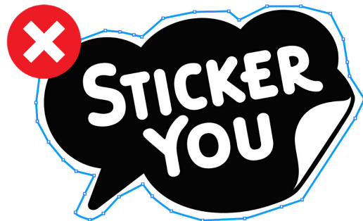
Does not adhere to the padding/safe zone requirement: too many anchor points, sharp acute angles with uneven spaces around art.
