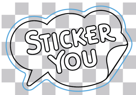
Working file example with substrate showing through and with areas with visible white ink in areas intended.
