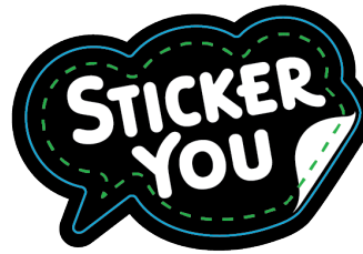
Example of a proper use of Bleed (8pt), diecut and content within safe zone (8pt)
